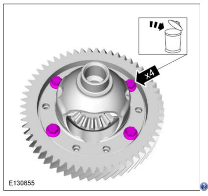
4. Tighten each bolt 1 turn at a time.
