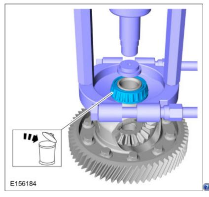
This side was a lot more challenging. What I ended up doing was removing the cage and rollers as with the other side. BUT I could not remove the race with my separator. What I did was use my Dremel to CAREFUL-LY cut a long, skinny notch on each side to slip the bearing separator into. DO NOT CUT THROUGH THE RACE INTO THE SHAFT! But do make the notch big enough for the puller to "grab" onto. After doing so, mine came right off.
