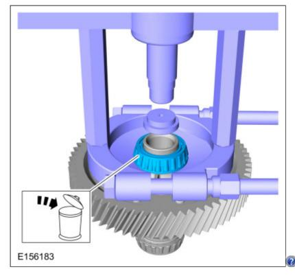
I cut the roller cages off and removed the rollers prior to doing this, as they just got in the way. Heavy nippers will make easy work of the cages. A bearing separator will be fine here on this side.
