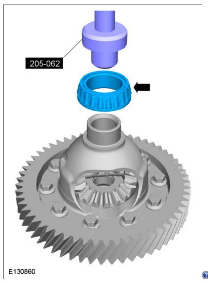
The special tool is not necessary, but DO be sure to ONLY press on the race and NOT the cage/rollers!! This is critical!! I used a large socket and some flat steel bar stock.
