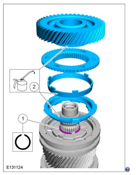
10. *Special Tool(s)* : 205-D015 (D80L-630-4) Step Plate *General Equipment* : Hydraulic Press All of these go in easily. Use lots of oil!
