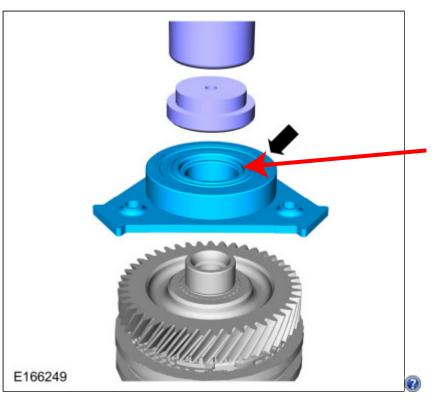
Be sure you are pressing on the inner race ONLY. I would recommend a socket that fits in the recessed area, as it does not go all the way down on the shaft. (will site a few thousandths proud) ALSO note the orientation of the bearing - the metal plate is DOWN.
