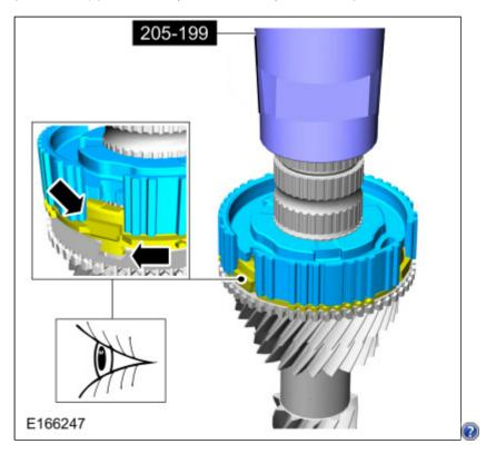
I didn't need the shaft installer here. All of these parts went on easily by hand and seated nicely. Take note that all of the tabs line up. Material : Motorcraft® Dual Clutch Transmission Fluid / XT-11-QDC (WSS-M2C200-D2)
