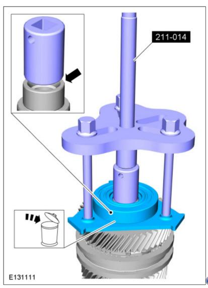
DO NOT try to remove this bearing with a simple three arm puller. IT WILL NOT WORK AND YOU WILL BEND THE METAL PLATE. You will need one of these "steering wheel" or "flywheel" pullers. I bought a set on Amazon and they worked like a charm.
