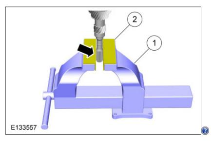
Make sure you have the plastic vice jaw protectors installed. Do not put your shafts into a vice that does not have jaw protectors installed! You'll screw up the shaft!
