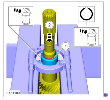
This race was fairly easy to get off with the puller. A good bit of area to bite onto. I did not use the press, but rather the bearing separator and the included puller arms and bolts.
