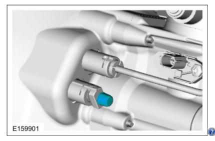
9. In order to remove any small amounts of trapped air remaining in the system, operate the clutch pedal 5 times, using the full clutch pedal travel.
